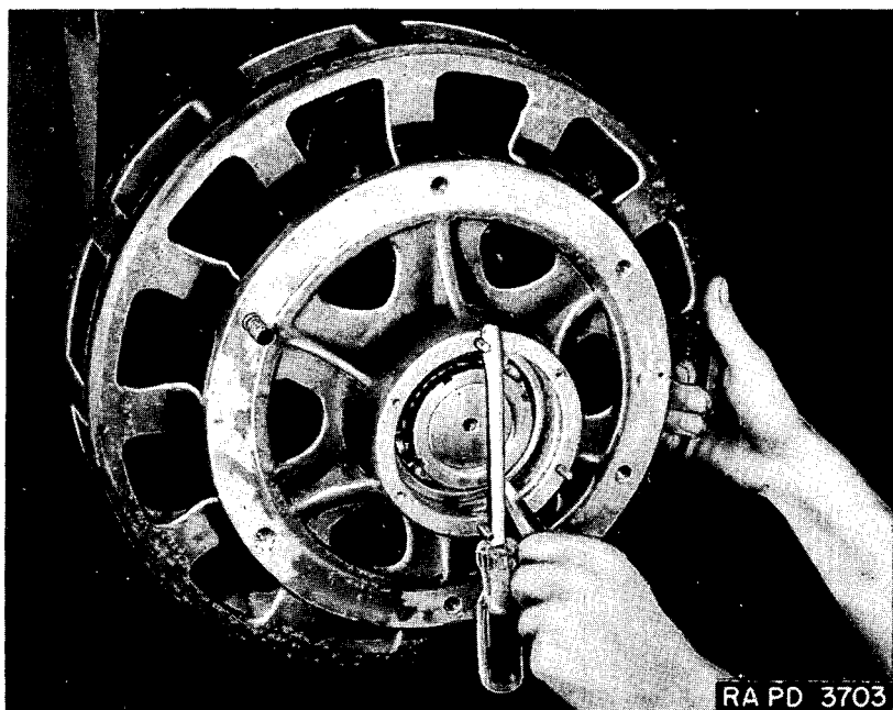
Figure 138—Removing Track Adjusting Idler Bearing Nut
