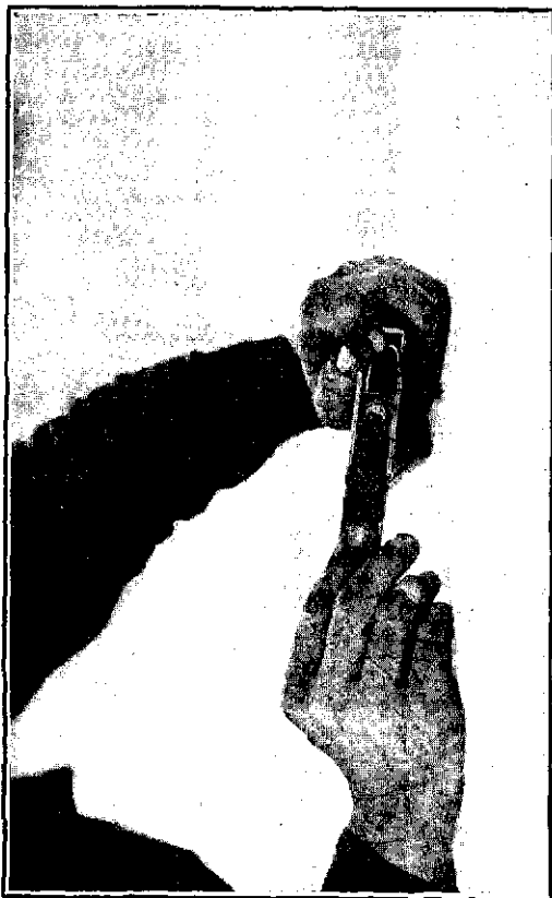
③ With left hand hold magazine spring in position. Slide magazine base fully home.
